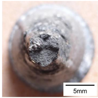
(1) Mold preheated at 350°C and coated base and work wash
